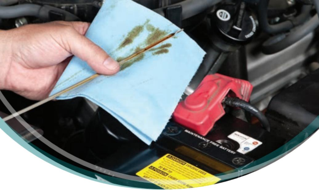
**Battery** The battery supplies power to the starter motor, acts as a voltage stabilizer and makes up for any shortfall when the alternator can't meet the vehicle's electrical needs. Inspect battery cable connections at every oil change and clean as needed. When inspecting a battery, always wear eye protection and gloves.
