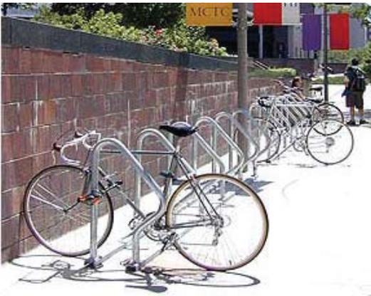
*Acceptable racks, like the “Post and Ring”, “U” racks and “Swerve” racks have two-point support and fit a variety of bicycle types.*
